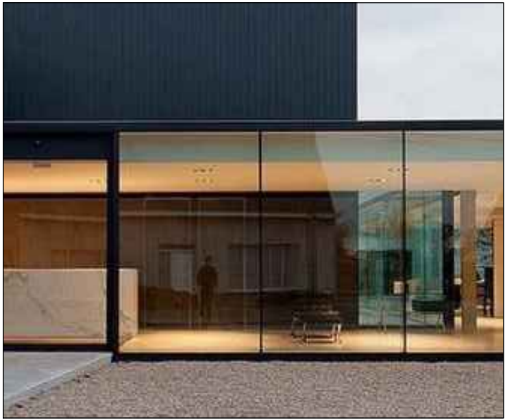
AFC ALUMINIUM FRAMED GLAZING DULUX DURATEC ETERNITY CHARCOAL PEARL SATIN OR SIMILAR
